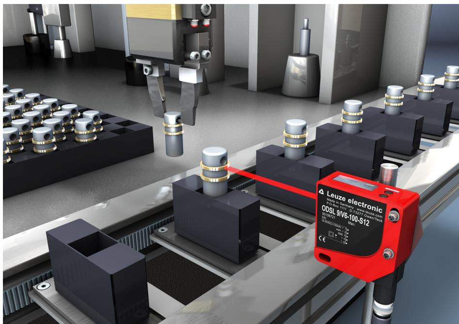
Fig. 4.2: Application example: assembly inspection
